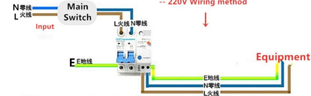
The neutral wire must be connected from the main switch to the air switch and then to the oven.
